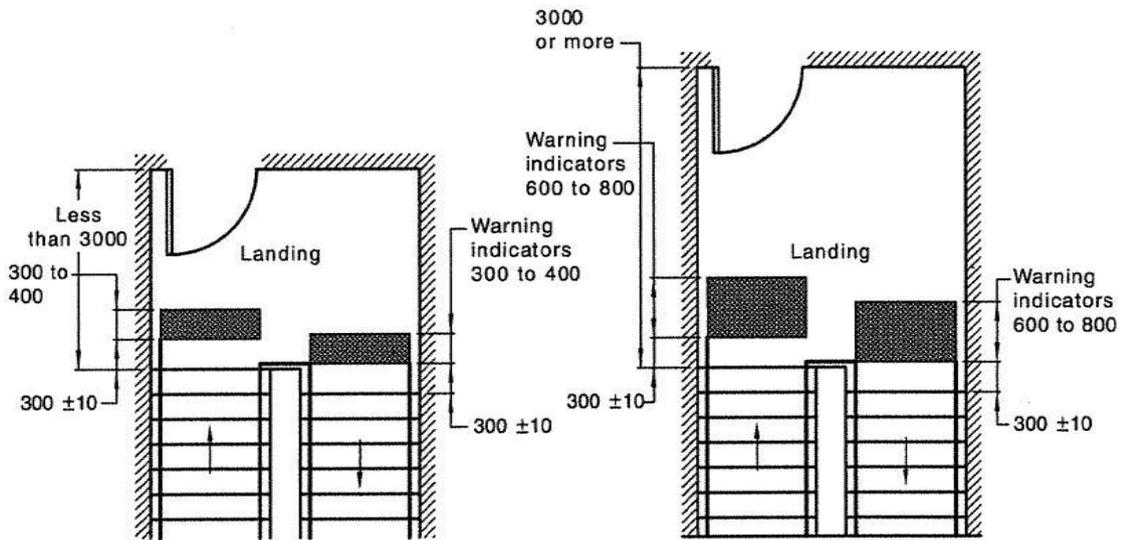
a) Stairway with landing less than 3000mm and no continuous outer handrail
